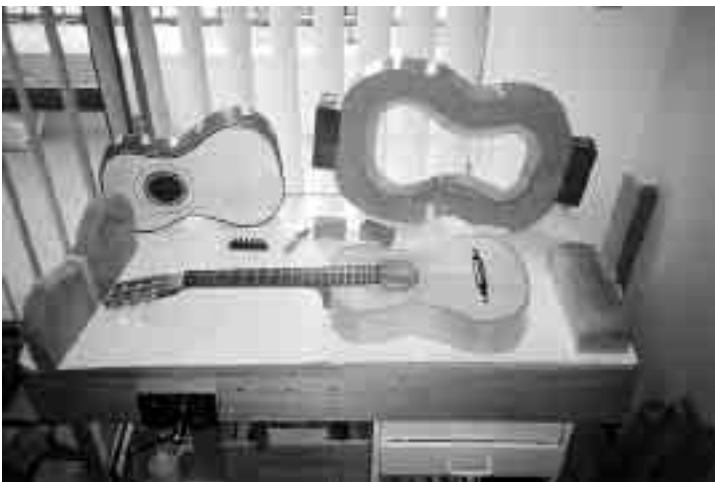
The completed instrument with some of the jigs needed to build it
